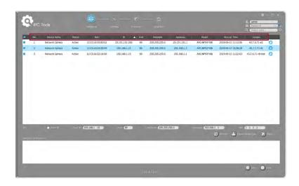
3. Select a camera or multiple cameras according to the MAC addresses; the camera must be assigned an IP address to be accessible.
