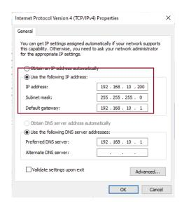
B. Click "Advanced", and then click "IP settings" > "IP address" > "Add". In the pop-up window, enter an IP address that is in the same segment with your Avycon IP camera (e.g. 192.168.10.200, but please confirm that the IP address you pick does not conflict with another address on the network);
